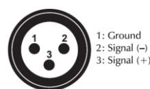
DMX-input XLR mounting-plug:
