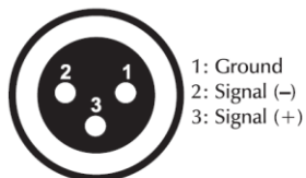
DMX-output XLR mounting-socket:
