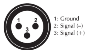
DMX-input XLR mounting-plug:
