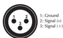
DMX-input XLR mounting-plug:
